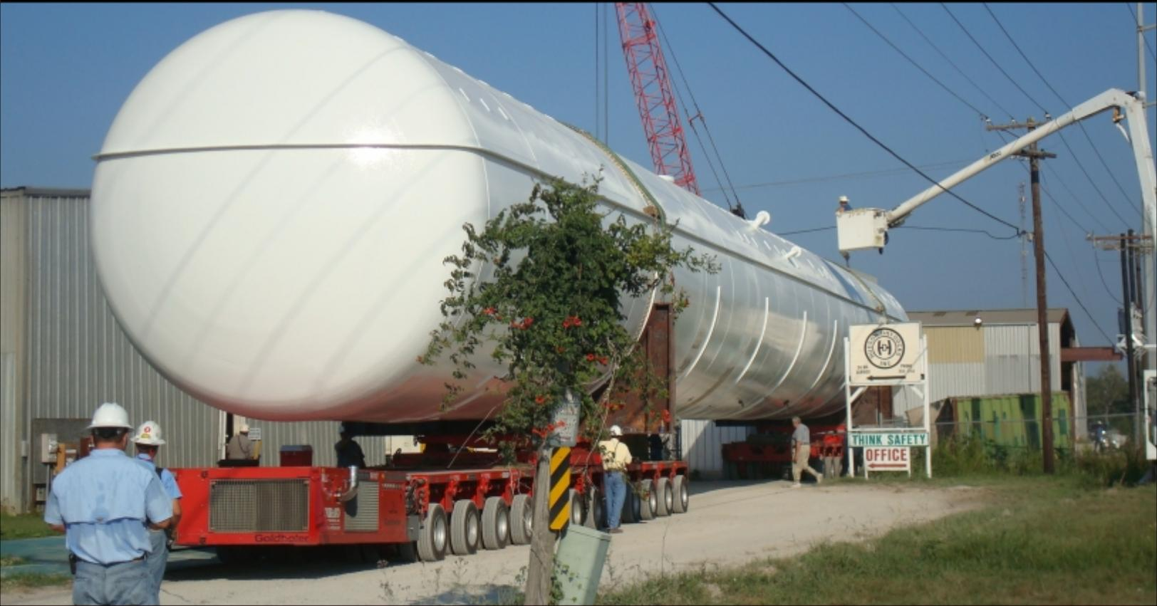
These two 200' x 17' 335 ton storage tanks were received from stands in a customer's yard and transported via city streets to an awaiting crane over a mile away. Berard provided detailed descriptions of transport path throughout the move, including detailed drawings showing exactly where matting would be needed, or where objects would need to be removed. Despite sweltering temperatures nearing 100 degrees, the people, equipment, and plan worked flawlessly in time and under budget.
